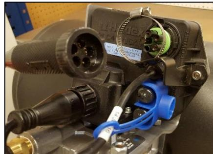
3. Inspect every light to be sure water hasn't infiltrated the housing. If there is water intrusion, replace them before reconnecting pigtails.
