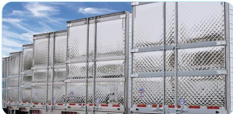
The bonded foam "sandwich" design of Utility's Barrier Door® and unique vinyl gasket seal, reduce weight and helps maintain temperature better than any other door design. The 3000R reduces heat transfer in another critical way too. A low conduction thermal break between the threshold and buckplate optimizes thermal efficiency and lowers reefer unit operating costs.
