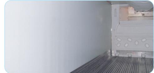
Utility's high impact lining is found on the complete interior—side walls, front walls, roof, and rear doors of the 3000R. This wards off damage from forklift impact, which reduces maintenance costs and minimizes the risk of heat loss, moisture, and pathogens getting into insulation.
