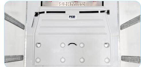
Removable air return bulkhead provides convenient access to refrigeration unit, making it easier to clean behind the bulkhead and the unit's coil, a common location for pathogen growth.
