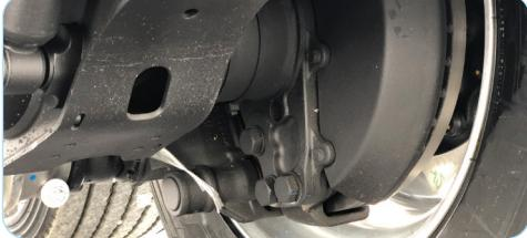
Disc brakes reduce brake fade, increase braking performance and improve safety—creating shorter, more stable stopping distances. With an extended service life, it lowers maintenance costs and downtime.
