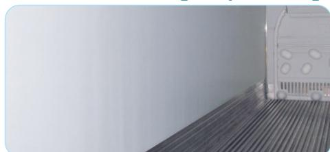
Additional thicknesses of high impact linings from multiple suppliers are available for severe service operations.
