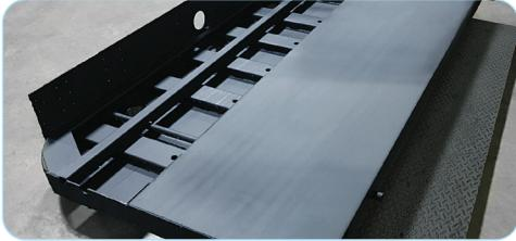
Engineered with a thicker approach plate and kingpin plate, this design minimizes damage during heavy-duty service operations, reducing repair costs.
