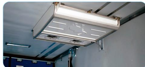
Factory-installed remote evaporators are available in a variety of locations for all multi-temp trailer requirements.
