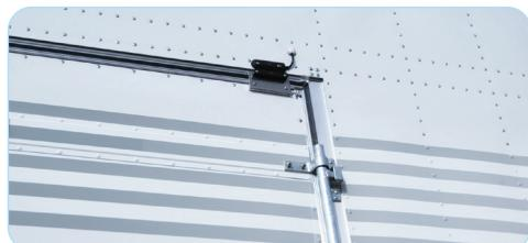
Shuts reefer unit off when an open door exposes the inside of the trailer to the ambient environment.
