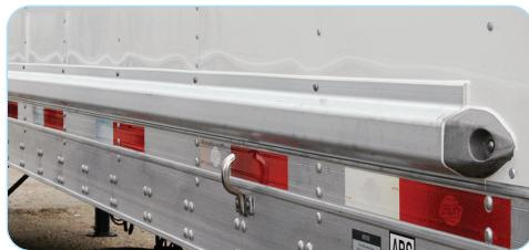
Constructed from heavy-duty aluminum, they protect the exterior side skin from casual damage, reducing maintenance costs.
