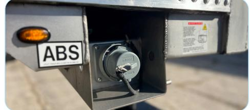
The advanced plug and wiring system delivers greater fuel savings during operation and improves safety with multiple grounding features.
