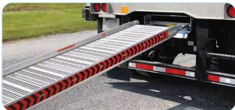
Most manufacturers' ramps are available for factory installation in both side and rear door configurations for greater ease in loading and unloading.
