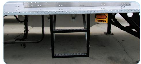
Available from most manufacturers in a variety of styles, side steps and rear steps improve operator safety and provide ease of accessibility.
