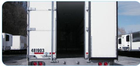
Barrier design is for tight clearance conditions in order to meet the need for a smaller door opening and lower heat loss.
