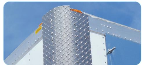
Aluminum diamond plate protectors defend against potential high clearance obstructions, reducing maintenance and repair costs and increasing trailer life.
