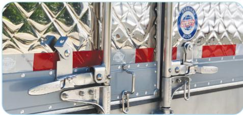
Electropolished stainless steel produces a corrosion resistant, easy-to-clean polished finish for improved appearance and increased resale value.
