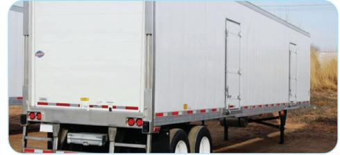
Doors can be positioned in a variety of locations in order to increase compartment accessibility and meet your specific requirements.
