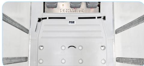
A number of air return bulkheads are available to fit a variety of refrigeration units. Several different styles of pallet stops are also available.
