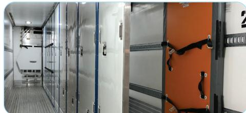
The thermally efficient CenterSeal load partition device allows for multiple zones inside a trailer for increased load versatility and efficiency.
